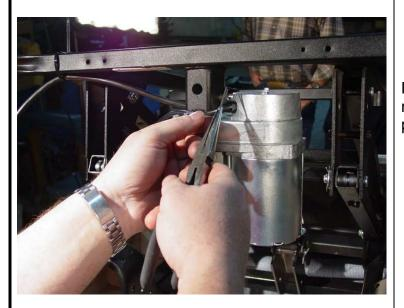
Replace the cotter pin into the steel pin and re-tie motor power motor cord to lift mechanism with a plastic wire tie.
