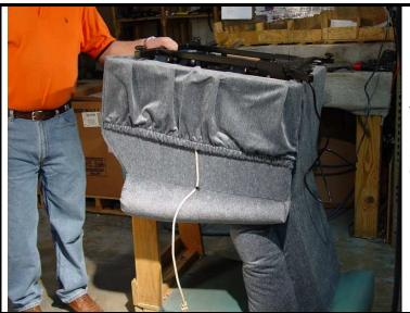
Unplug chair from wall outlet and turn the chair over to allow access to the underside of the chair.
