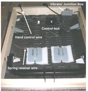
Zip tie the control box to the seat springs as far back to the seat frame as possible. Note the location of the wiring. Seat vibrators begin and the spring retainer wire.
