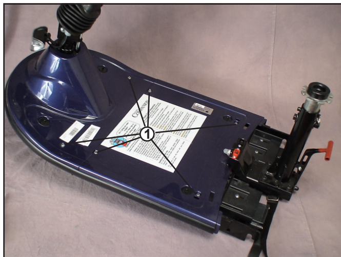
Figure 30. Floorboard and Front Shroud
