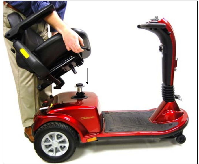
FIGURE 24. REINSTALL THE SEAT
