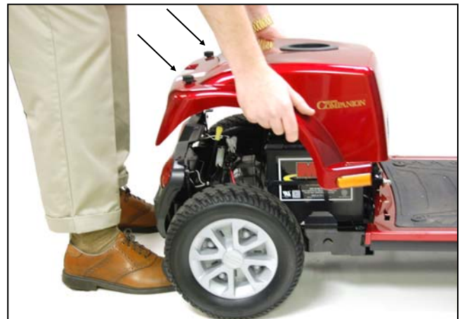
FIGURE 16. REMOVING THE REAR SHROUD
