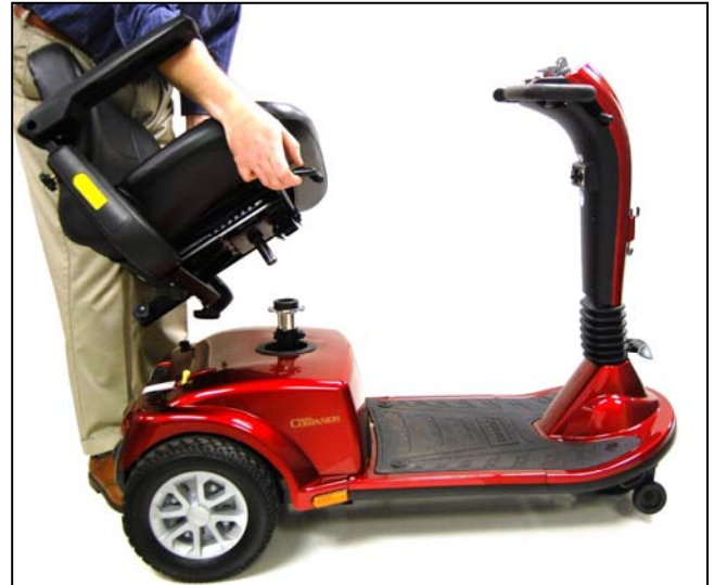
FIGURE 15. REMOVING THE SEAT
