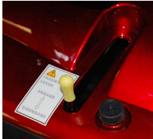
FIGURE 12. FREEWHEEL LEVER (DISENGAGED)
